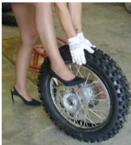
The slick way to get the tire off the rim—remove the first side then half the second side, stand the tire up and push the rim off with your high heels.
