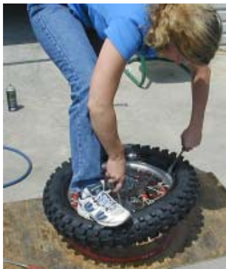
Lever the first bead down onto the rim, then taking two or three-inch bites lever the rest of the tire on.
