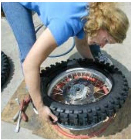
Pull out the tube, get the valve in, then dig down and capture the rimlock with the bottom tire bead. Put the valve stem nut on so you don't lose the stem.
